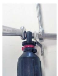
Step 4 Attach the lever arm to the PR500 Bracket using the 5/16"phillips head machine screw and self locking nut. Use the white nylon washers on each side of the bracket. Tighten securely, but not too much. The handle should rotate with minimal force.
