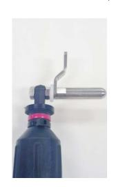
Step3 Hold the lever arm handle with a 7/16" wrench and the 5/16" hex bolt with a ½"wrench and tighten well. Note: Insure that the actuator can rotate freely, but remains snug.
