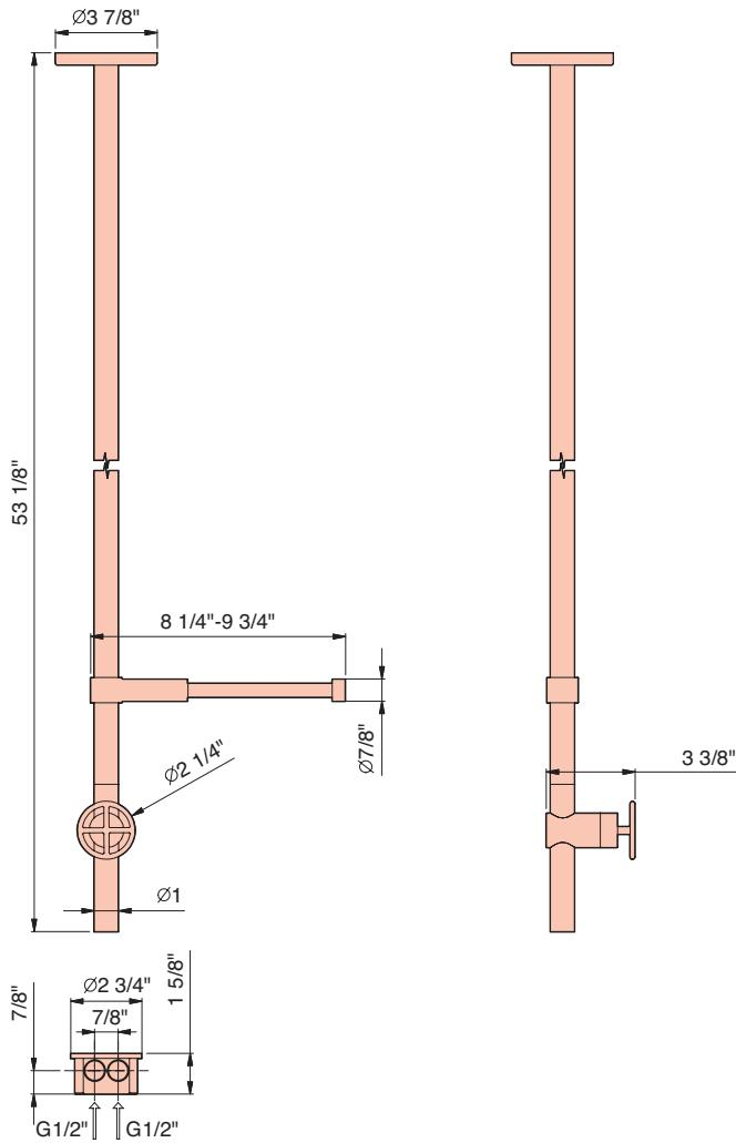
**EN** These mixers can be used with high-pressure hot water accumulators or with instant water heaters.
