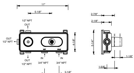
**EN** These mixers can be used with high-pressure hot water accumulators or with instant water heaters.
