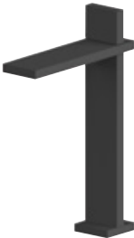
ART. T006WU Single-hole vessel mixer, 5 3/8" spout projection / Progressive cartridge. Mitigeur lavabo surélevé monotrou, entraxe bec 5 3/8" / Cartouche progressive. Monomando lavabo alto, distancia a chorro 5 3/8" / Cartucho progresivo.
