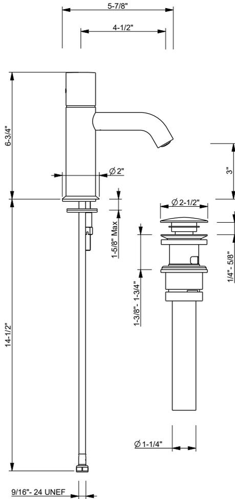
**EN** These mixers can be used with high-pressure hot water accumulators or with instant water heaters.
