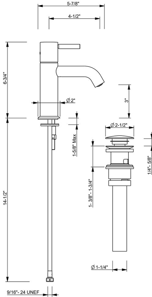
**EN** These mixers can be used with high-pressure hot water accumulators or with instant water heaters.
