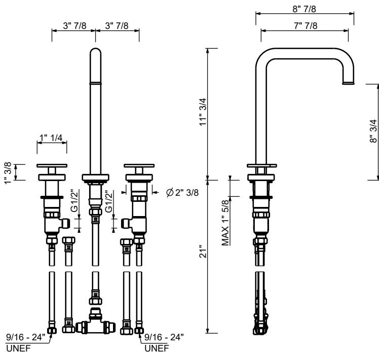
**EN** These mixers can be used with high-pressure hot water accumulators or with instant water heaters.
