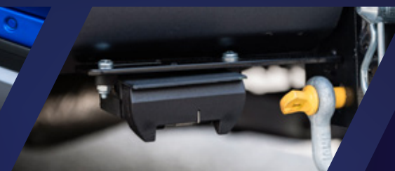
◀ Towbar pack includes 7 pin flat connector
