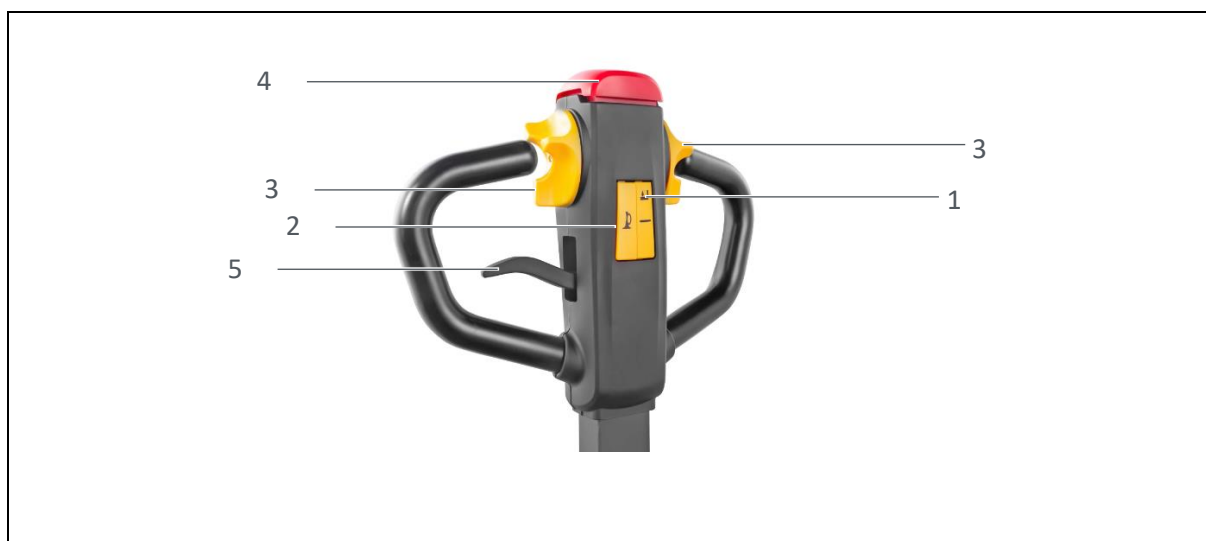
Fig. 12: Main components of the drawbar
