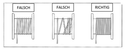
Leave at least three turns of the cable on the reel to avoid stressing the cable and damaging the cable's connection point.
