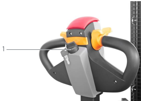
Fig. 11: Ignition lock on the rear of the drawbar
