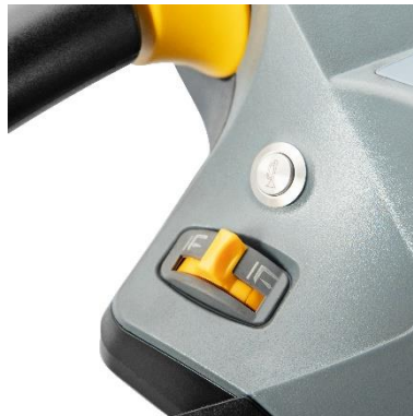
Fig.19: Switches for lifting and lowering on the drawbar
