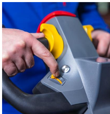
Fig.20: Hand position when lowering the load
