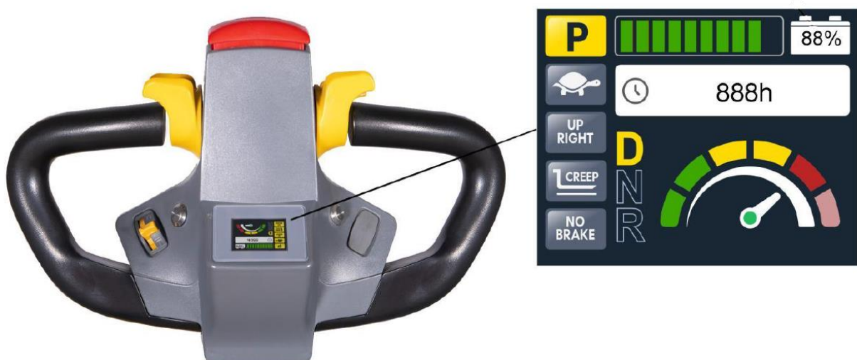
Fig.8 : Tiller with display
