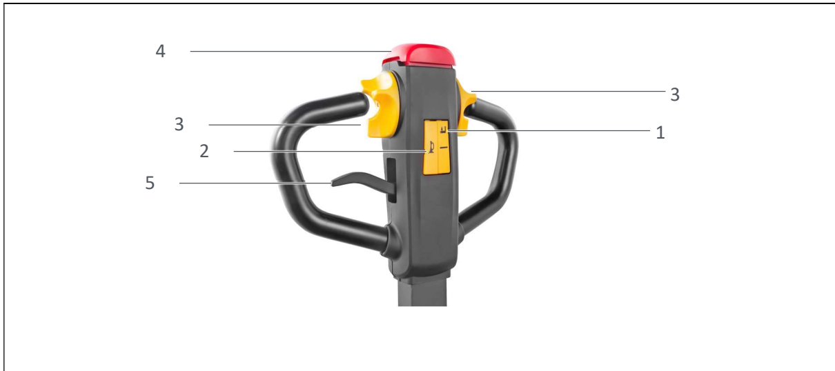
Fig. 4: Main components of the drawbar (front and rear)
