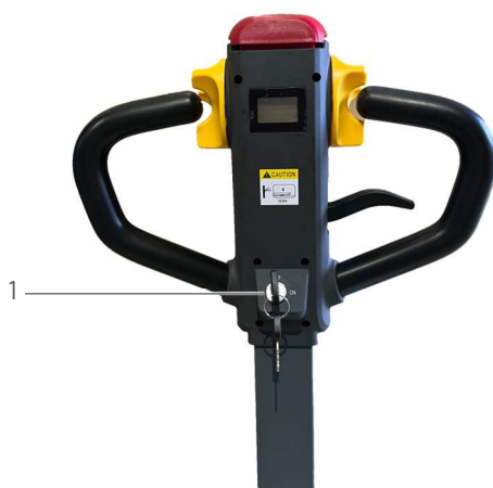
Fig. 9: Ignition lock on the rear of the drawbar
