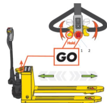
Fig.38 : Activating travel with the tiller in an upright position
