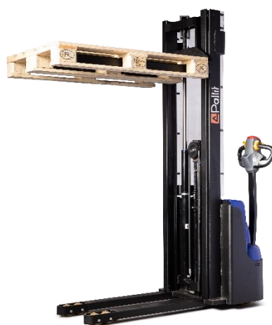
Fig.11: Fork in top position with free lift
