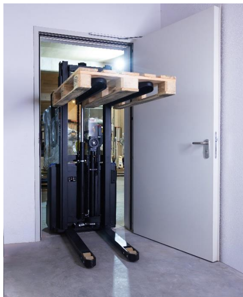
Fig.22 : Example of a driving situation with free lift
