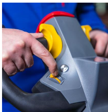
Fig.20: Hand position when lowering the load
