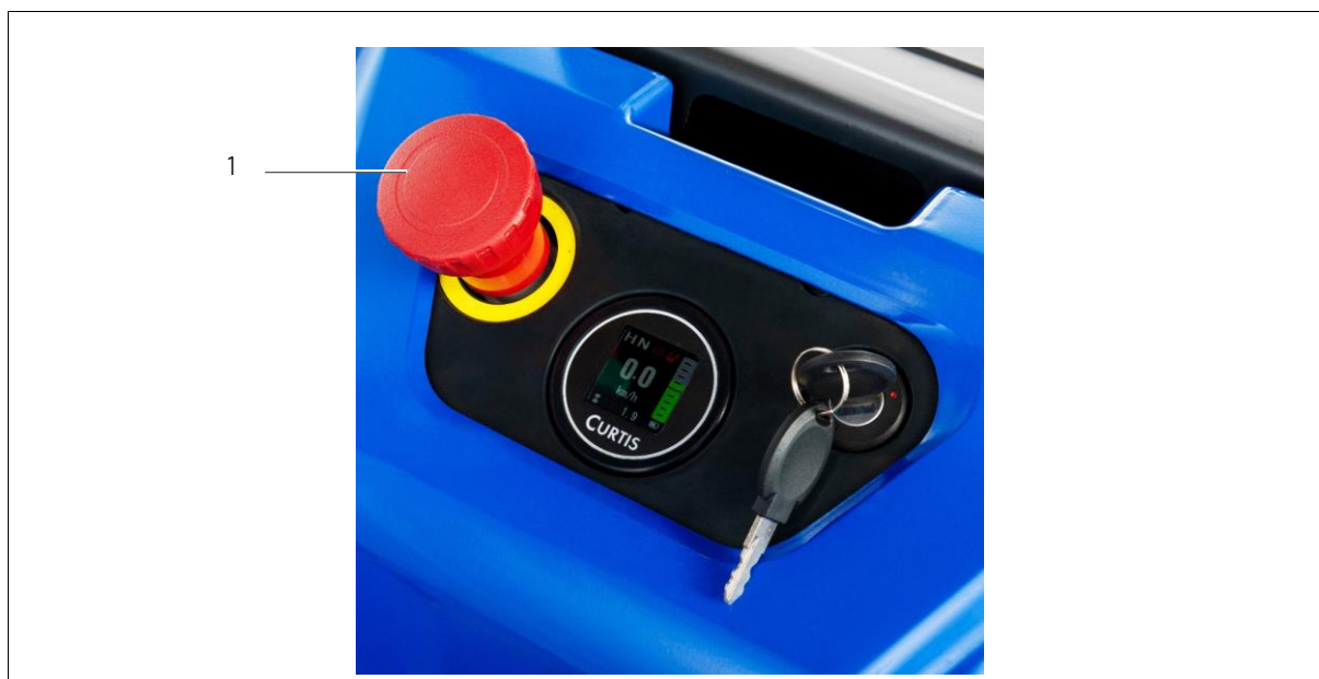
Fig. 1: Emergency stop switch
