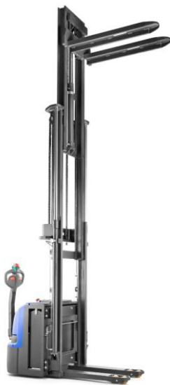
Fig. 11: Fork in top position
