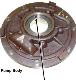
**Step 3** To prevent front seal blowout, Enlarge this hole 1/4" to 9/32".
