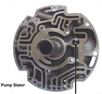
**Step 4** Under "X" drill a 3/64 (.042-.055) hole thru side of wall in direction of arrow.
