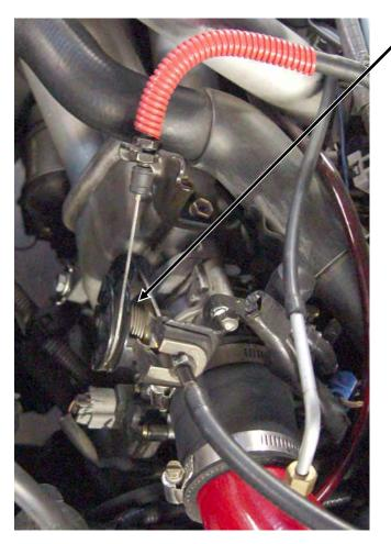
**Step 3** Verify TV cam moves about same time as the throttle opens. Adjustment is same as the stock setting.
