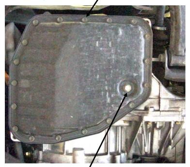
Tighten drain plug to 30 FT LB
