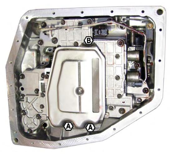
**Step 2** Remove filter bolts "A" and "B". Identify bolt lengths **Page 3.**
