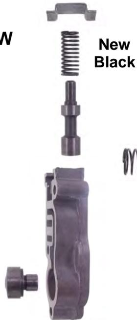
**Step 2** Remove original 1-2 spring and install **NEW Orange** spring.
