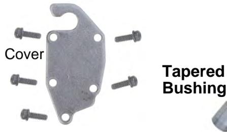
**Step 2** Install Tapered Bushing into hole. With long VB bolt, drive bushing into hole about 1" down. It's not fussy. Reinstall cover.
