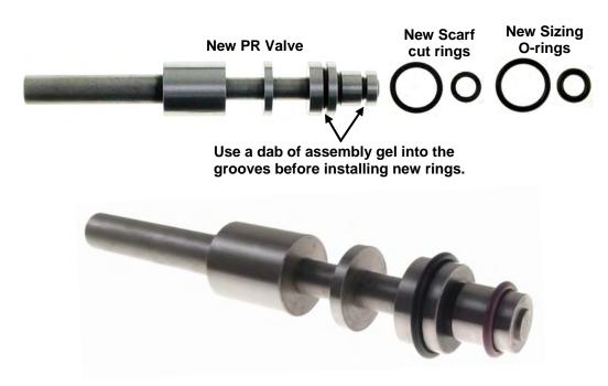
New PR with New Rings and Sizing O-rings installed. Put it in the freezer until ready to insert it into VB. Remove sizing O-rings just BEFORE installing Valve.
