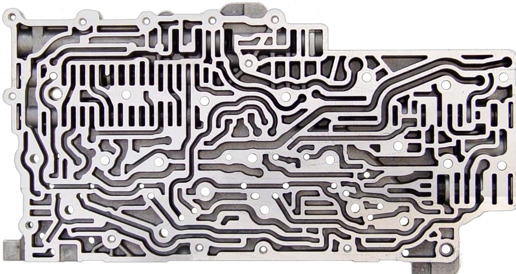
**2.** Clean the bore thoroughly. Then try the valve by itself in the bore first to ensure it is moving freely. Install **new compensator feed regulator valve**, original spring, and retainer.
