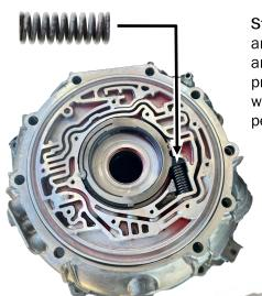
Step 1. Install pump slide and pivot pin by removing and discarding original priming spring. Replace with the **new** white high performance priming spring. Step 2. Remove and discard original pump vane rings and install the new unbreakable rings.
