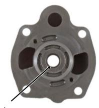
Check pump shaft bushing
