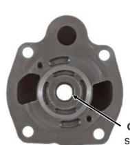
No raised boss or machined hole here is JF011E. It is a higher volume pump.
