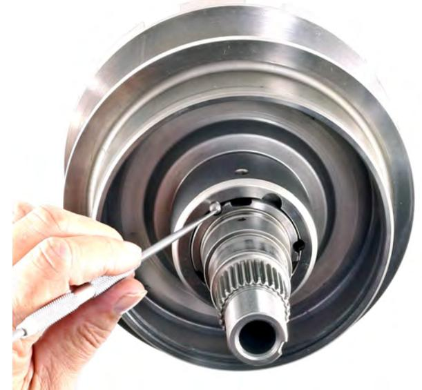
It may be necessary to push each ball into the groove with some light pressure. Do not use a hammer! A little pressure and wiggling of the sheave and they will go right in.
