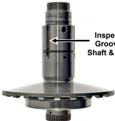
Inspect Ball Grooves on Shaft & Sheave.
