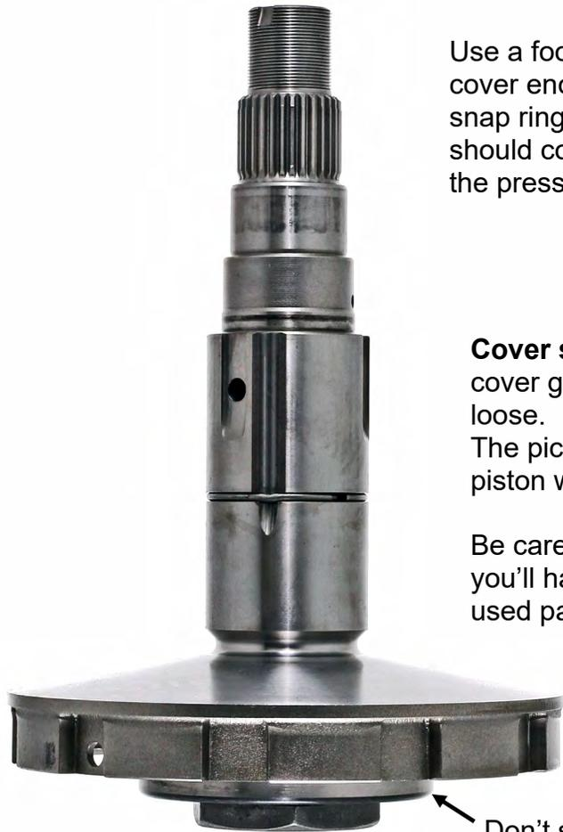
Use a foot press to press down on the piston cover enough to release the pressure off the snap ring holding the cover on. The piston cover should come out of the sheave as you release the pressure on the cover.
