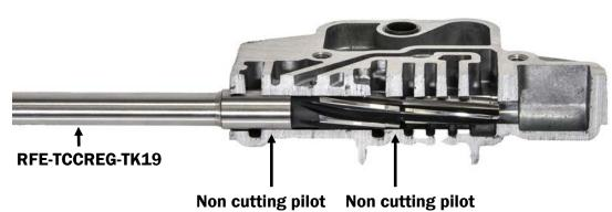
**3.** Using lots of WD-40® and **low speed** on your favorite portable drill, let the reamer do the cutting until it bottoms in the bore. Don't force the reamer. Bore finish and reamer life require a slow inward movement and lots of WD-40®.
