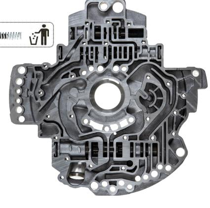
**4.** Once reamed, clean the bore and the new TCC regulator valve furnished in this kit. Test fit to make sure the valve is free in the bore. Lube and install the **new TCC regulator valve and new spring** followed by the end plug and retainer clip.
