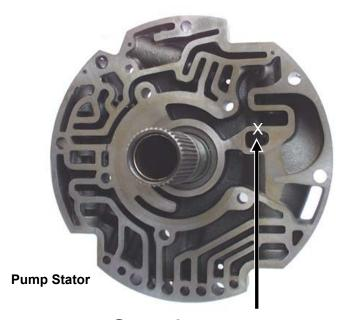
**Step 1** Under "X" drill a 3/64 (.042-.055) hole thru side of wall in direction of arrow.
