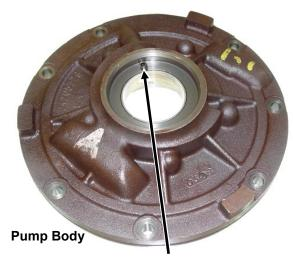
**Step 2** To prevent front seal blowout, Enlarge this hole with 1/4" drill.
