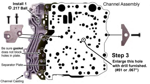
Install one check ball © in Channel Casting.
