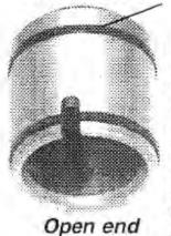
Install expander wire with ends towards you. Then install the seal with ends away from you. Before inserting into bore make sure the angle cut ends of the ring fit together and wire is under ring. © TransGo 1996
