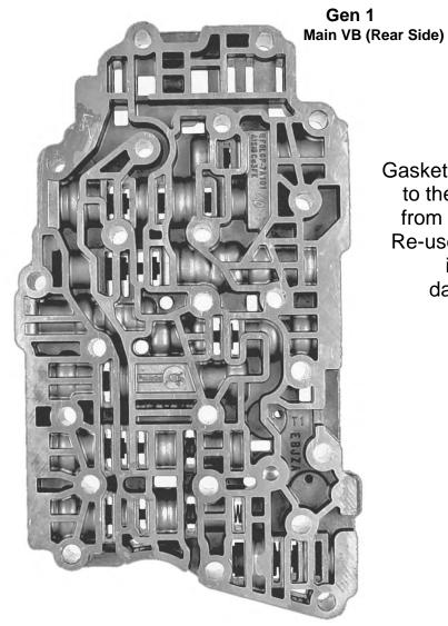
Gaskets are bonded to the rear plate from the factory.
