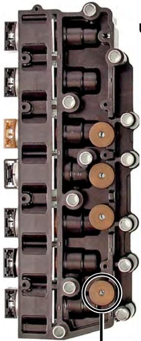
Use a small amount of assembly gel to hold the parts in place before putting module side onto solenoid side.
