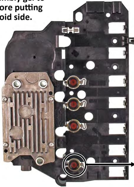
Corner of Razor blade works best to remove old diaphragms.
