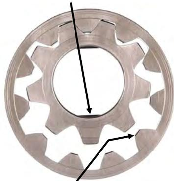
Beveled Edge on outer gear teeth faces converter!
