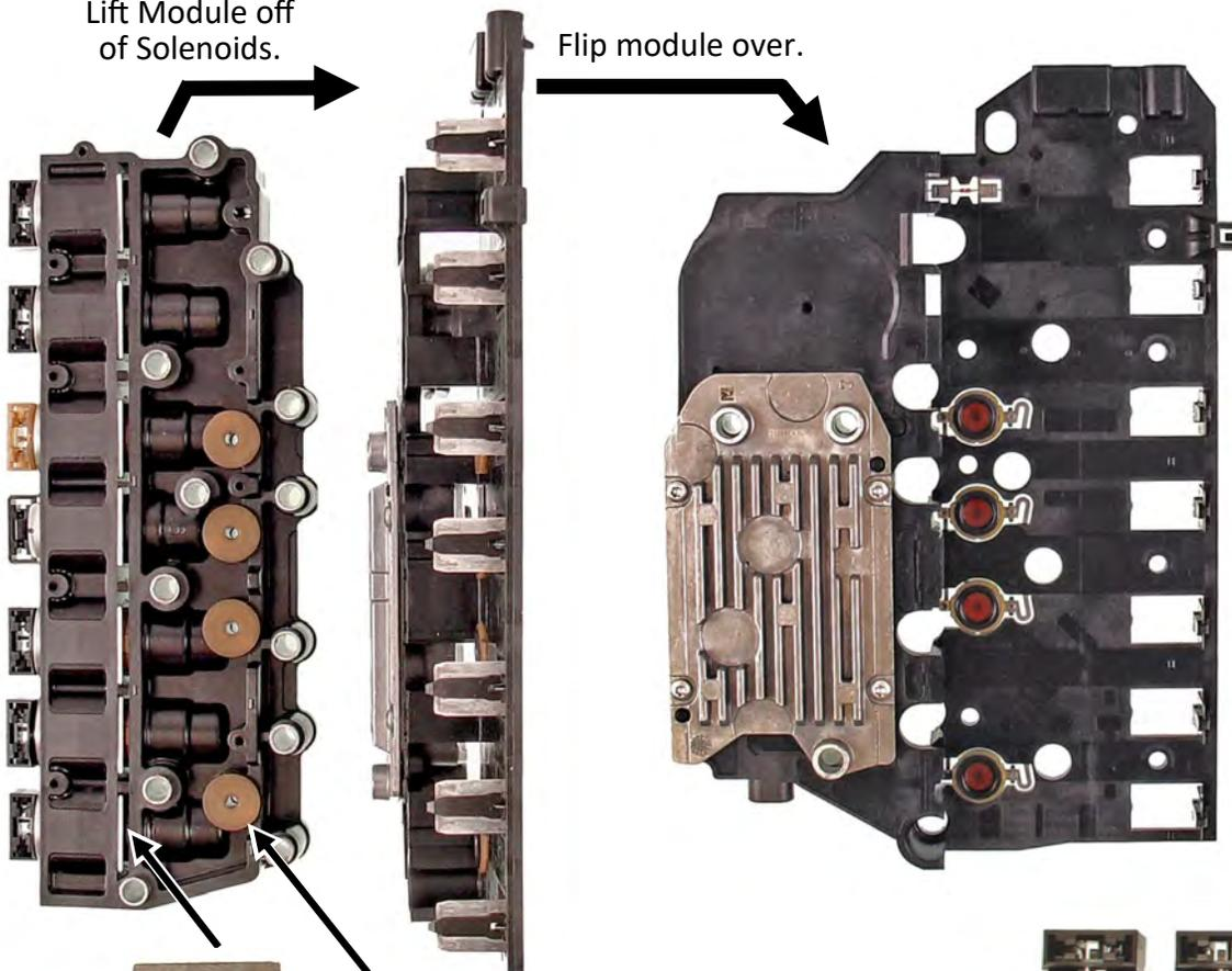
Remove 1 solenoid at a time, clean the solenoid, lube seals & re-assemble with original retainer.
