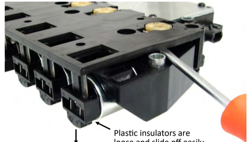
Slide plastic downward to re-install insulators.
