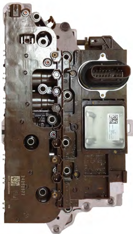
TEHCM (Front View)
