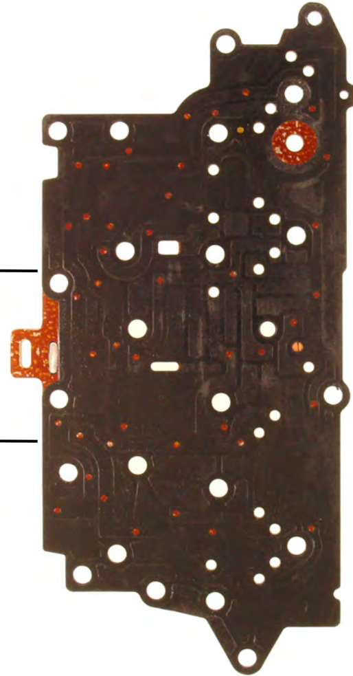
Front Steel Cover Plate (Rear Side) w/Bonded Gasket
