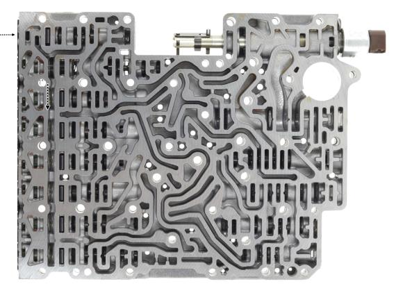
**7.** Reinstall the solenoids back into their original locations, then install the retain plate and the 9 #27 Torx<sup>®</sup> bolts, torquing them to 70 lb·in.
