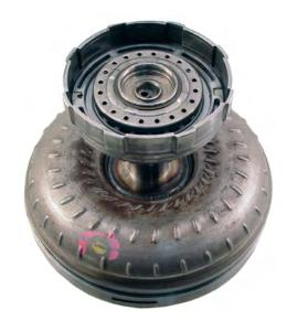
Always insert the input shaft into the converter till it bottoms out. Lift the drum up gently and you'll feel the seal lightly dragging on the shaft which feels different from the spline drag. No feel? Look into converter and inspect the seal. The shaft must have drag on the seal or you risk a TCC performance issue!
