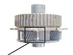
**B** Find the lube hole just above the bearing. Drill a ¼" hole through a clutch groove in line with the lube hole. Then enlarge the lube hole to ¼". Lube hole.
