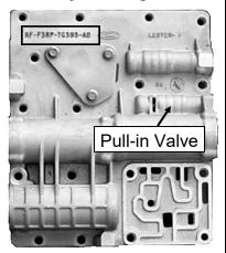
93-96 Casting # starts with "RF-F3" and has a "Pull-in Control Valve".
