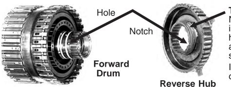
This Picture: Notice the bushing is welded to this hub due to misalignment of the splines.
