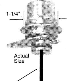
Pin: Diam 3mm [1/8"]. Length: 1-3/16" to 1-1/4" Install flat end of capsule into hole.
