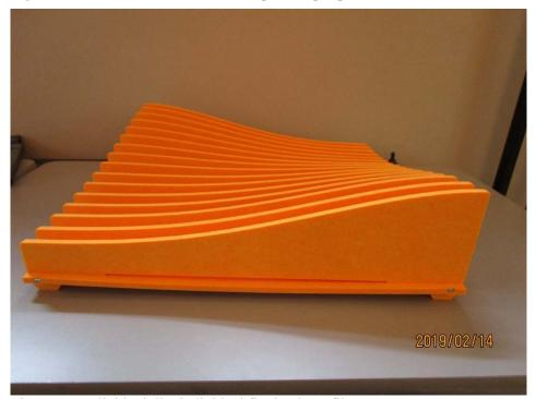
Figure 4 – Individual tile, individual fin depth profile
