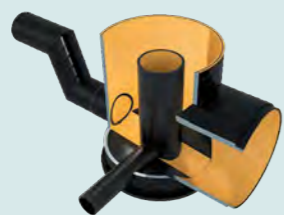
Manhole intake with overflow pot and roughing
