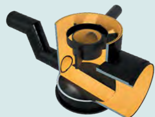
Manhole intake with inside drop/drain pipe
