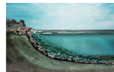
Active capping of sediments
