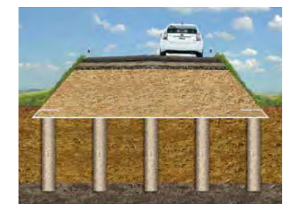
Geotextile Encased Columns
