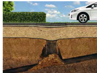
Bridging of Sinkholes
