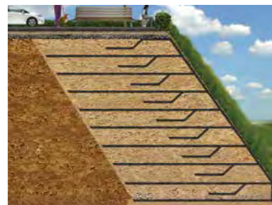
Geosynthetic Reinforced Soil
