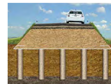
Geotextile Encased Columns (GEC)
