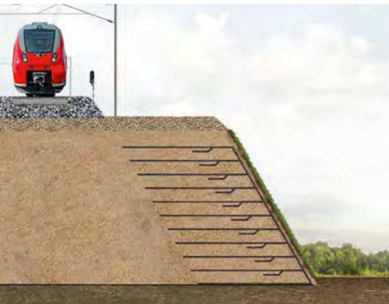
Retaining walls/steep slopes
