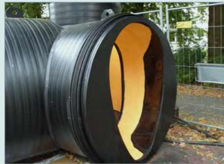
Transition to oval profile with welded haunch made of PE plates with tight-connection wall integration
