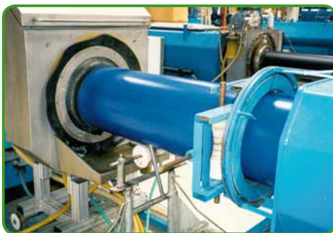
Fig. 14 - Extrusion plant for pressure pipes at AGRU-FRANK GmbH
