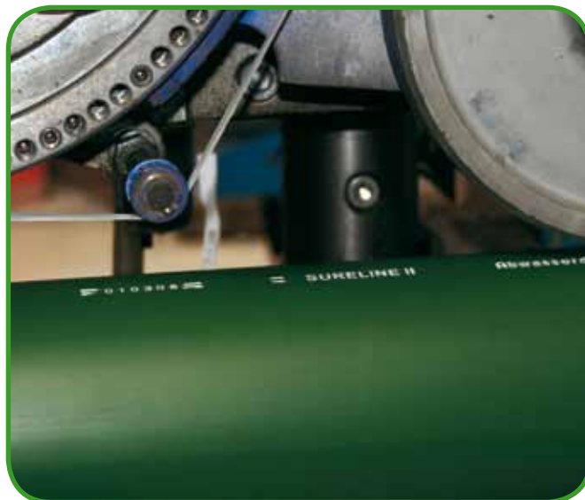
Fig. 29 - Identification mark on extruded sewage pipe
