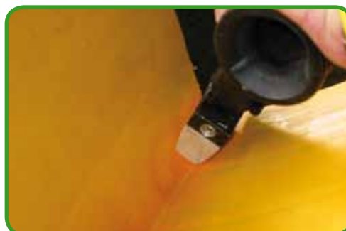
Fig. 110 - Extrusion seam/welding seam
