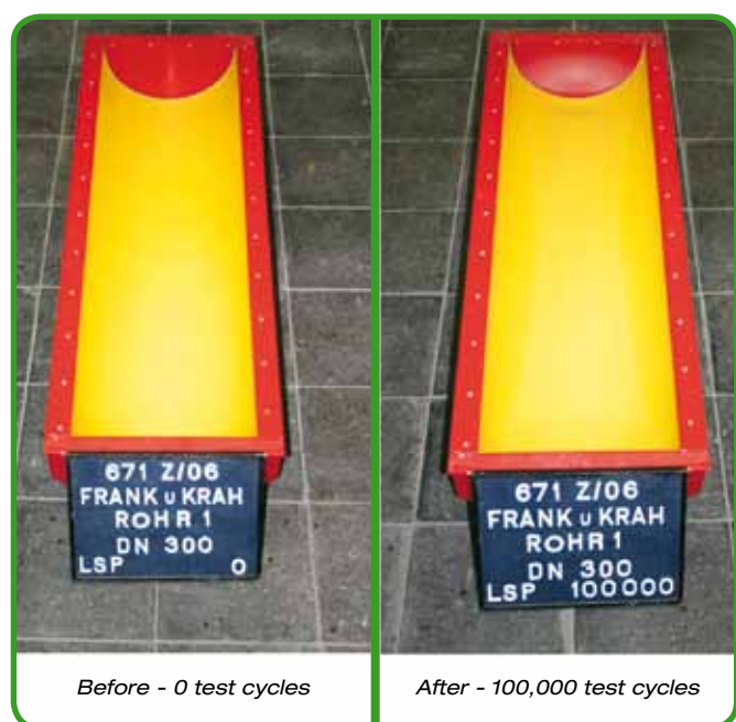
Fig. 59 - PKS® pipe (PE 100), DN 300 in abrasion test, FRANK & KRAH Wickelrohr GmbH
