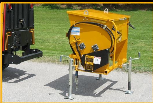
The Rear-Mount Sidewalk Spreader was specifically engineered for sidewalk applications. By dispensing a 41-inch spread width, it is designed to avoid the waste and turf damage often associated with broadcast type spreaders. The delivery roller further conserves material by spreading it evenly in a diamond pattern rather than a solid layer. Making efficient use of the spread material will allow you to go farther, prolonging the need to return for a refill saving material, labour and fuel costs.
