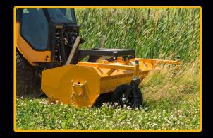
The Trackless front-mount Flail Mower was designed to cut heavier grass, weeds, scrub and light brush where a conventional rotary lawn mower could not cope. An enclosed mower housing and rubber safety skirts keep the cut grass, mulch, and other debris within the cutting chamber and enable safe mowing near roads, parks, and other busy or populated areas.
