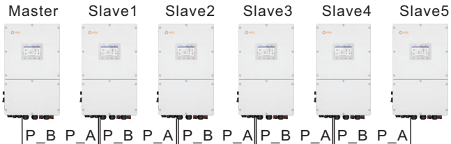
Figure 3.22 Parallel Terminal Connection
