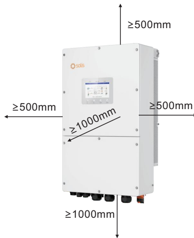
Figure 3.5 Inverter Mounting Clearances
