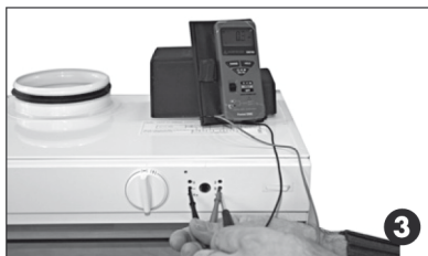
Measure voltage at contacts – and S, adjust for instance speed 1 at potentiometer 1.
