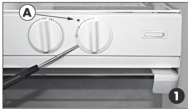
Set the speed knob in position 1 and detach the knob with for instance screwdriver.
