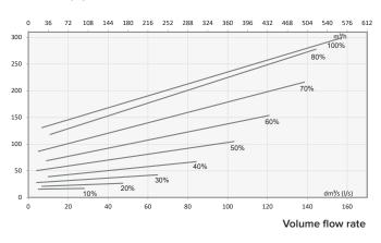
Pressure loss in ducts. Total pressure (Pa)
