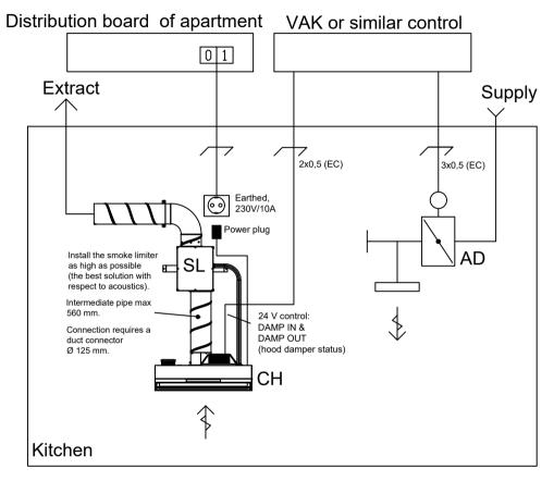
In order to carry out maintenance and adjustment, there must be access to the Adjustment Damper, e.g. a maintenance hatch.
