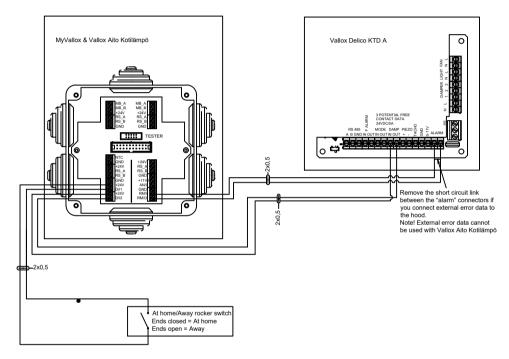
Select At home/Away as the setting used for the digital input 1 and Programmable input as the setting used for the digital input 2. Set the desired supply and extract air fan speed for the Programmable input and select a suitable supply air temperature. Set error message, maintenance reminder, both, or off as the relay function.
