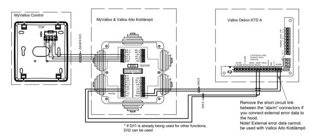
Select Programmable input as the setting used for the digital input 1. Set the desired supply and extract air fan speed and select a suitable supply air temperature. Set error message, maintenance reminder, both, or off as the relay function.
