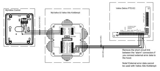
Select fan speed control as the function of the analog input. Set error message, maintenance reminder, both, or off as the relay function.
